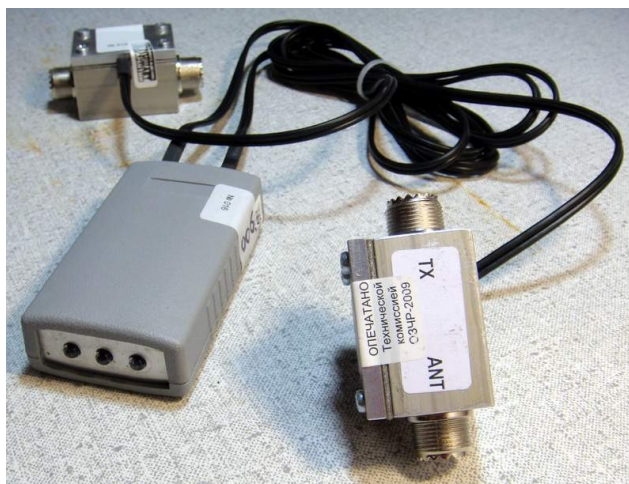
Fig. 1 – WRTC-2010 peak power monitor: LED indicator module (at left) and two coupling/detector heads.
